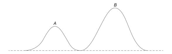
The heights of *A* and *B* above ground level are 20 m and 22 m respectively. The length of the track between *A* and *B* is 16 m. The resistance to motion of a biker on the track may be modelled by a constant force of magnitude 50 N. The total mass of the biker and his bike is 70 kg. The speed of the biker at *A* is  $v \text{ ms}^{-1}$ . Find the minimum value of *v* if the biker is to reach *B* without pedalling. [7]
